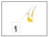
It's possible to connect a tag line at the rear in order to orient the evacuee when arriving at the ground.
